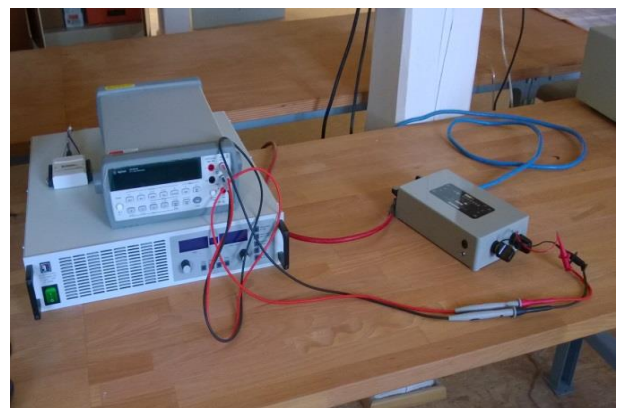
Figure 4 Error Determination with Reference Resistor
